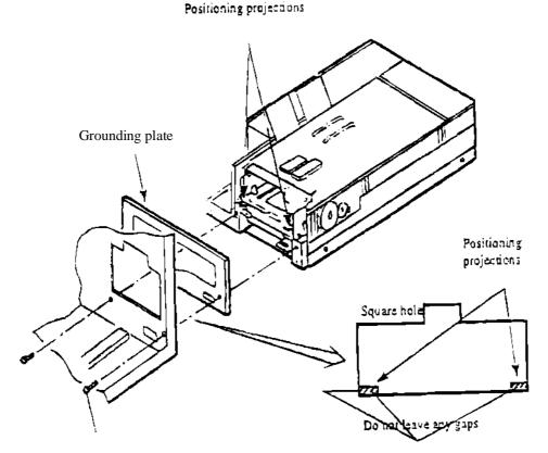
Figure 1-29. Connect the M2488 and the FACL
